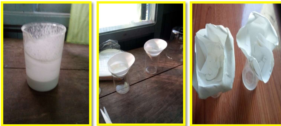
Figure 7. Al doped TiO 2 sample precipitate on flask, filter and dry in air for 120 hours
