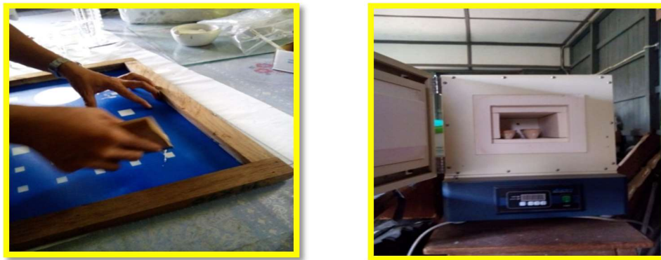
Figure 5. Sample deposition process by the screen printing method and heat treatment at different temperatures
