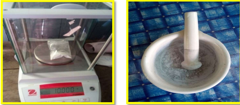
Figure 3. Weighing of chemicals with digital balance and grinding with aggregate mortar
